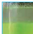
Refrigerant and additive contaminated by water
